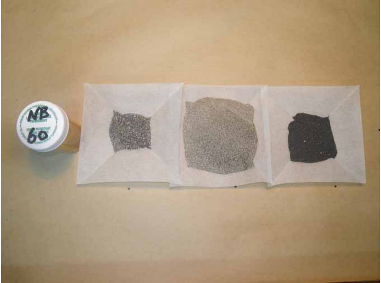
NB – 60 showing all four fractions ( Re Pan Con in the Vial, Plus 300Micron fraction, Re Pan Reject fraction, Pan Con Magnetic fraction)
