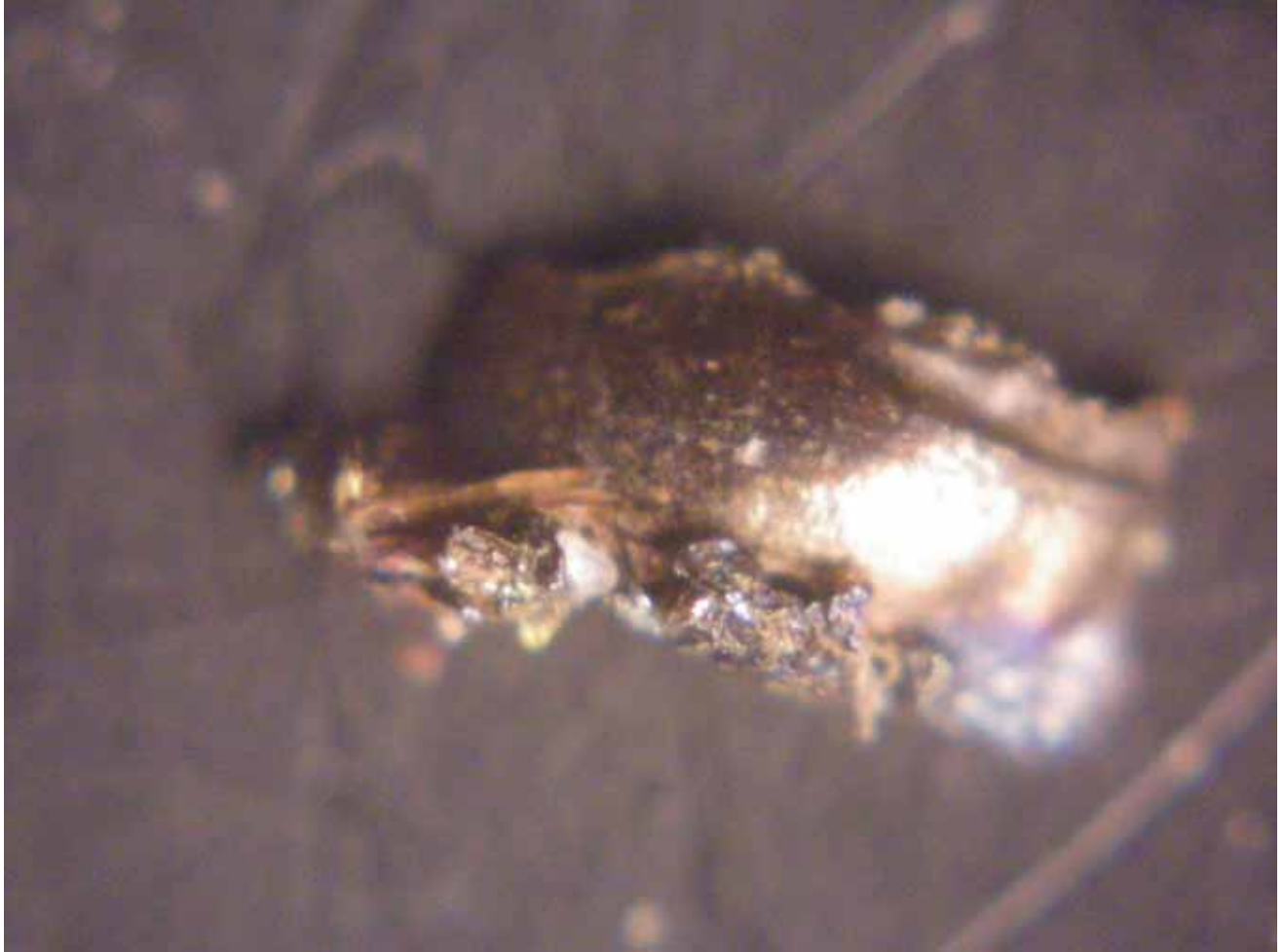
NB – 60 Pan Con fraction – Side 2 of pristine unidentified metallic nugget. Approximate size 145 x 60 microns.
